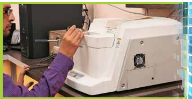
Thermogravimetry Tg Analysis (Resin System Process Control)
