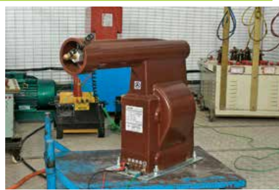
33kV PT test in operation
