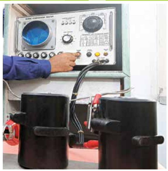
Switching Impulse Test
