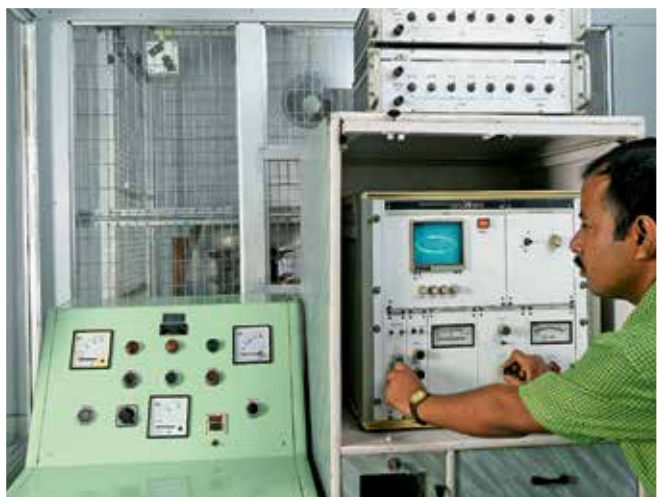
Partial Discharge Test
